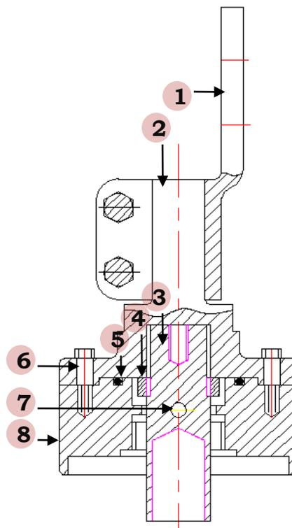
Fig. 8 Structure of the Bushing Head
