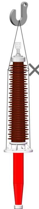
Fig. 6 Wrong Lifting
